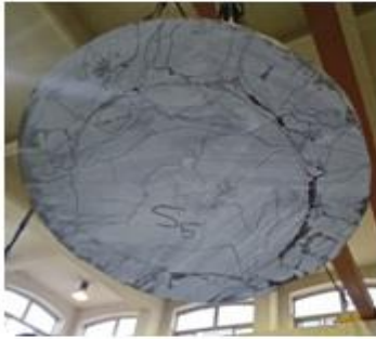
(a) Experimental crack pattern for S5
